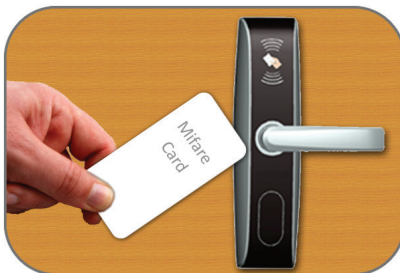
Tap the Mifare Card on the Door Lock to open the door
